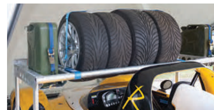
Tyre rack + fuel storage + work bench. (option). *check suitability of race or saloon car.
