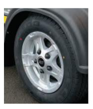
O Alloy wheels TUV approved, light weight 12" alloy wheels with safety locking wheel bolts.
