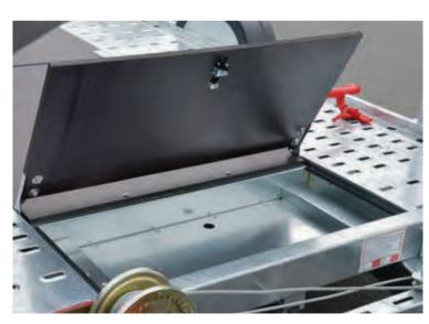
• Storage bed locker (front) Lockable front storage locker, with automatic lift lid.
